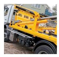
Rear hooks and torsion tube make loading and unloading speedy and safe
