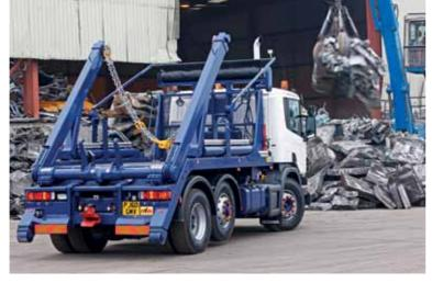
Skiploaders working in metals usually operate at higher GVWs. TITAN skiploaders are available in a full range of floor lengths to suit every type of truck chassis.
