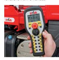
TITAN can be supplied with both TRR and manual lever controls
