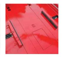
Fully bolted rear end speeds maintenance and reduces downtime
